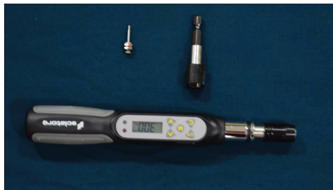
Figure 5: Digital screwdriver SP series with adapter and hex drive
