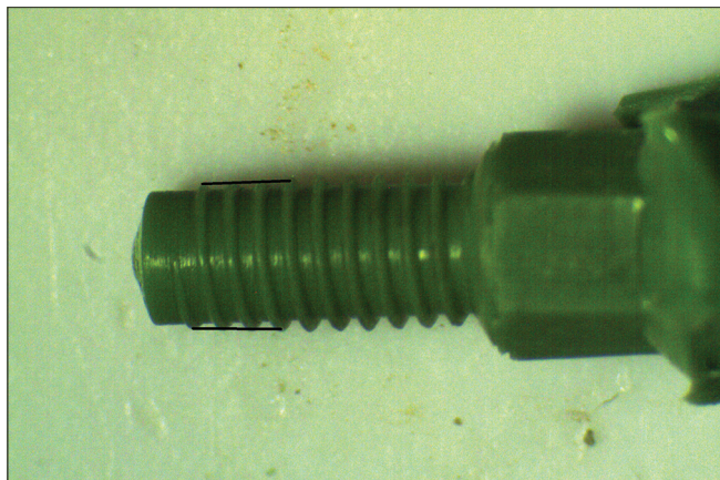
Figure 4: Distance between four threads measured using Biowizard software
