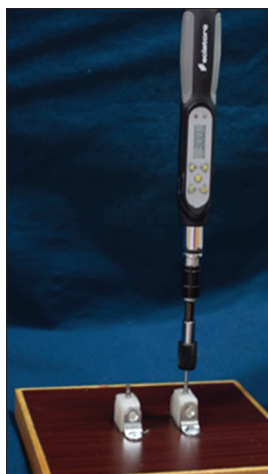
Figure 8: Measurement of torque using digital torque driver
